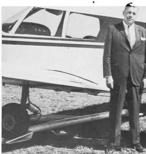
ANTI-SQUALL PHI Edmund L. (Skip) Eveleth (Brown '32) stands in front of a light plane anchored with his invention, an anti-squall device that holds light aircraft safely in high winds. It's called the Safe-T-Mount. ■
