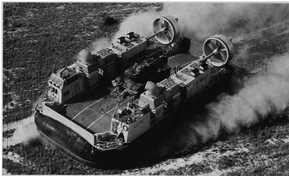
LANDING CRAFT: Bell Aerospace Textron is a pioneer in air-cushion technology and produces for the U.S. Navy the LCAC-1, an amphibious assault land craft.
